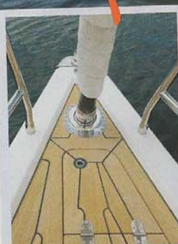
Roller up On deck, all hardware is flush, including the roller-furling unit that is installed below deck.
