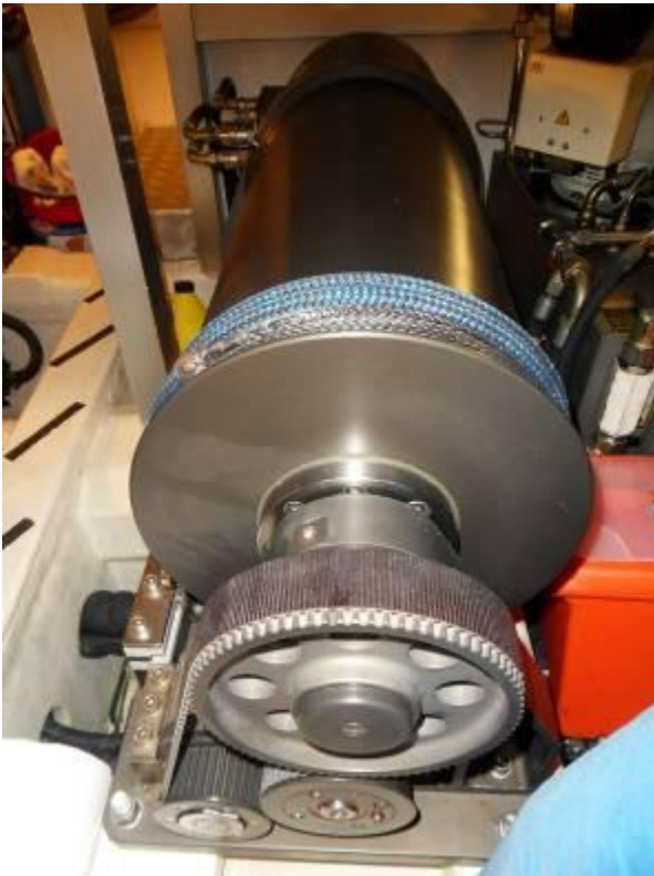
Captive main halyard winch in engine room and fuel valve chest
