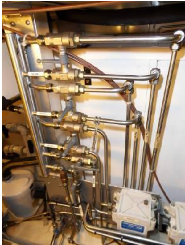
Captive main halyard winch in engine room and fuel valve chest
